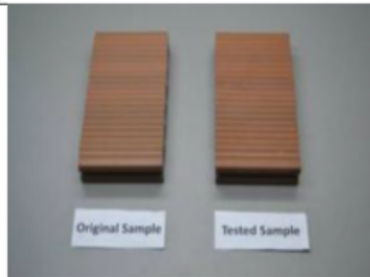
After 3000 hours test, Grey Scale 3, \Delta E^* = 3.64
