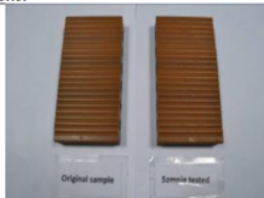
After 1000 hours test, Grey Scale 4-5, \Delta E^* = 1.41
